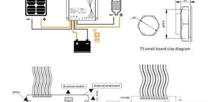
Wiring sequence: Firstly connect the load, then the battery and finally the solar panel.
